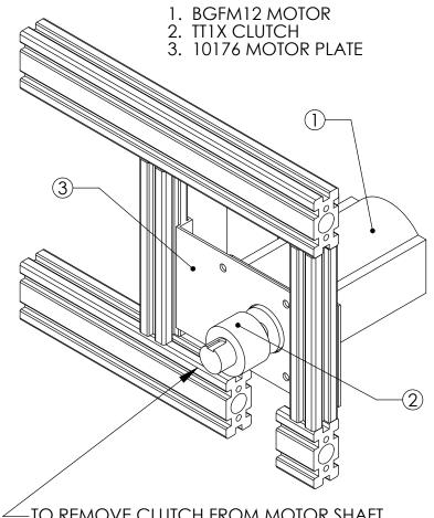
TO REMOVE CLUTCH FROM MOTOR SHAFT, LOOSEN (2) SETSCREWS WITH 3/32" ALLEN WRENCH FROM BOTTOM SIDE. ONE SETSCREW IS MATED WITH SHAFT FLAT.
